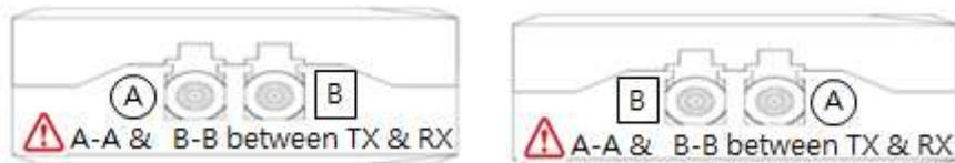
Fig Figure 3 – Fiber numbering & Caution on both fiber ports
