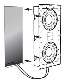
2. Screw in the six clamp screws. As the screw turns clockwise, a clamp rotates out and presses onto the back of the sheetrock to hold the subwoofer firmly in place. Tighten the clamps so they are snug, but do not over tighten, as they could damage the sheetrock.
