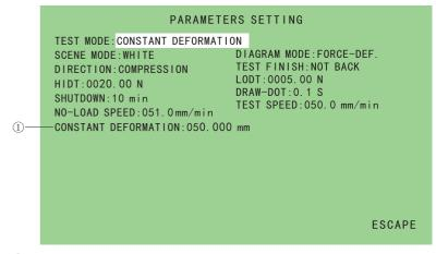
①Constant deformation: the spring tester will stop once it reach to pre-set deformation.
