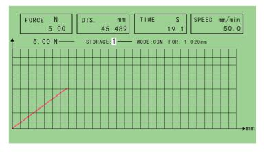
(Note: Under test interface, pressing "stop" button make the instrument stop testing amd enter curve storage interface)
