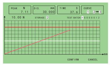
(Note:adjust cursor by "♠" "♥" "♠" buttons, and modify test batch, then save curve to corresponding place which the "♣" point by pressing confirm button and cancel save operation by pressing cancel button, return to interface of curve storage.)
