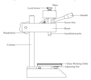
Note: Mass dimension: Ø64×31mm; Weight: 0.75±0.05kg; Installation pole size for connecting durometer: M7×0.5mm.
