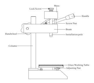
Note: Mass dimension: Ø55×8mm; Weight: 50±5g; Installation pole size for connecting durometer: M7×0. 5mm.
