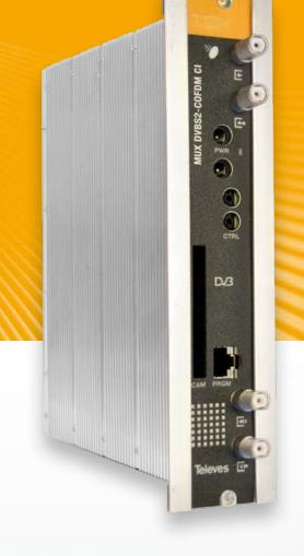
This is a device capable of delivering a Multiplex whose content is made up from services coming from different TVSAT transponders
