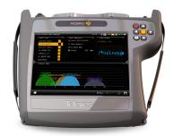
This functionality performs a comprehensive analysis of the entire Wi-Fi band (2.4 and 5 GHz), to find, identify and measure all available Wi-Fi networks. For this, MOSAIQ6 offers 4 different analysis functions:
