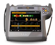
Connect the input signal to your MOSAIQ6 and within a few seconds the meter will automatically capture the signal. The device first searches for the standard and then for all the standard's parameters.
