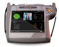
Allows the demodulation and analysis of IPTV streams (both Unicast and Multicast), not only through video display but also by displaying the total bit rate and the relevant information for each service: SID, VPID, AID, video profile, bit rate for both audio and video
