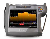
Professional spectrum analyser with ultra-fast digital processing (sweep time < 10 ms) and high dynamic range (> 50 dB). Equipped with advanced functions for the detection and analysis of signals in the 5 MHz to 3,300 MHz (waterfall, event triggers, markers, user configurable RBW and VBW, etc.).
