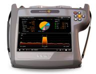
This function allows you to demodulate a DAB channel, providing signal quality measurements such as MER and CBER, and comprehensive information about the services delivered: Radio info: (Ensemble, PTY, Service, Mode, Audio- , bit rate audio). It allows power measuring between 20 dBµV and 128 dBµV, C/N and MER for this type of signals.
