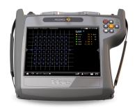
The constellation diagram is essential to help detect the presence of noise, phase jitter, interference and other potential problems that could impact the signal quality by reducing MER.
