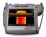
Signal levels turn into colours and are represented on the time axis (see figure). The perfect tool for short signal interference or fading analysis, which observation would be difficult by only resorting to the spectrum.
