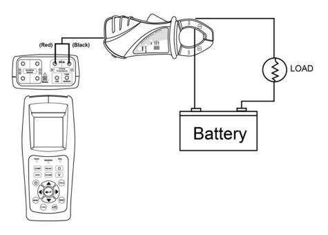
1. Connect the current probe to meter :
