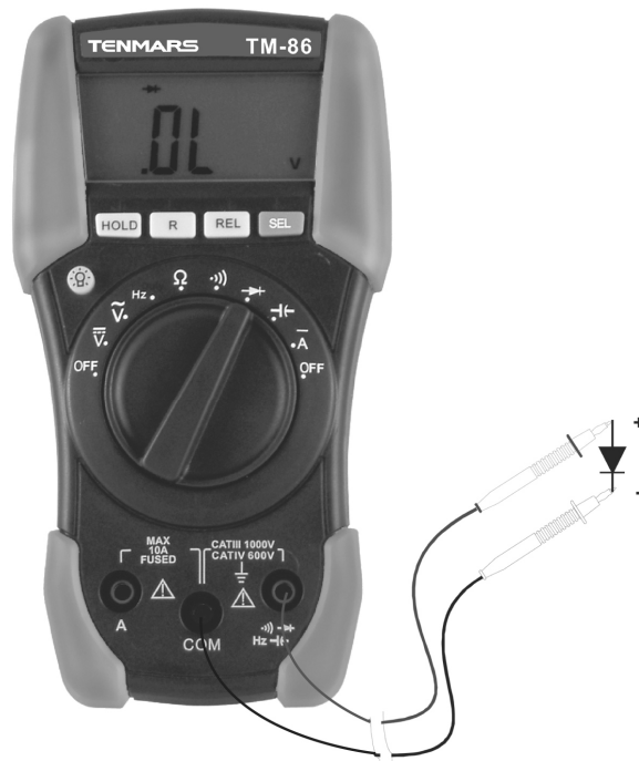
Fig. 8: Using the instrument for Diode test
