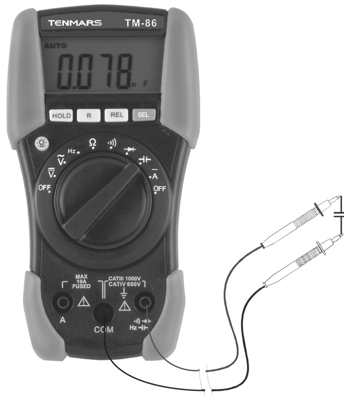
Fig. 11: Using the instrument for Capacitance measurement
