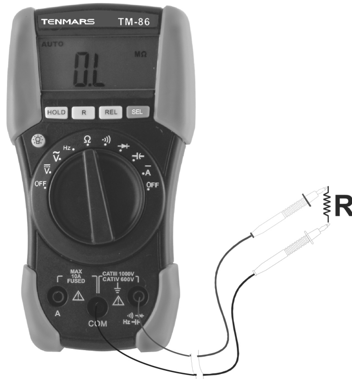
Fig. 6: Using the instrument for Resistance measurement
