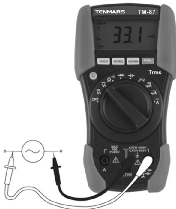
Fig. 3: Using the instrument for AC Voltage measurement
