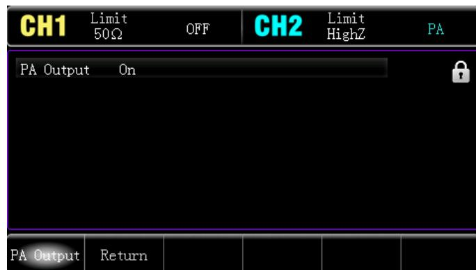
The weight power bandwidth of built-in power amplifier can output up to 100 kHz, the maximum output power 4 W, and output slew rate greater than 18 V/ $\mu$ s.
