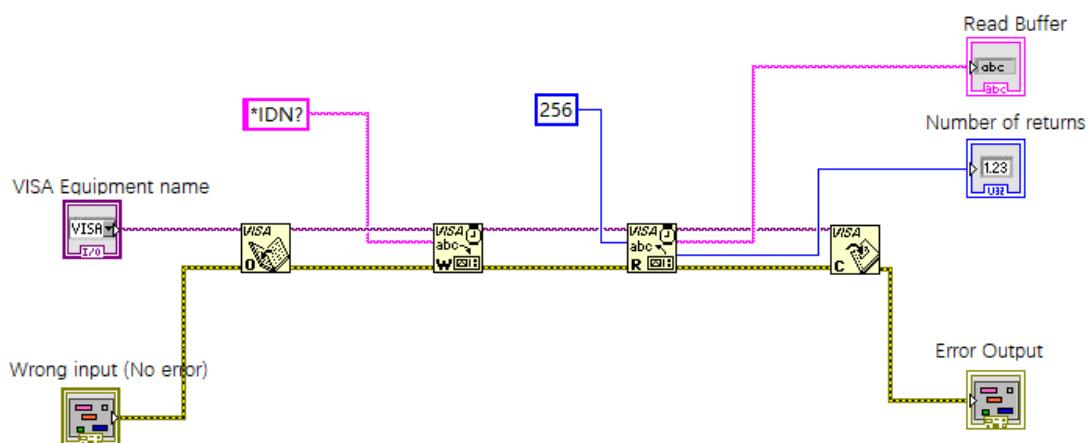
5. Communication with the device via TCP/IP is similar with USBTMC, it need to set VISA write and
