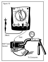
The MAP sensor is used to change a pressure signal into a DC voltage or frequency one. All GM, Chrysler, Honda and Toyota use DC voltage type MAP sensors, while Ford uses frequency type MAP sensors. Refer to relevant manuals for other automotive manufacturers. Testing Procedure:
