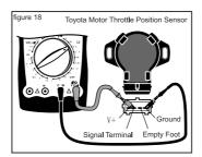
The position sensor is an electrometer or variable resistance. It is used for the computer monitoring of the position and direction of a mechanical device. The typical position sensors include throttle, exhaust recirculating EGR, blade air flow and other sensors.
