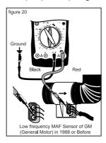
The sensor converts the air flow into a DC voltage, low frequency or high frequency signal. UT105 can only be used to test a DC voltage or low frequency signal. Testing Procedure:
