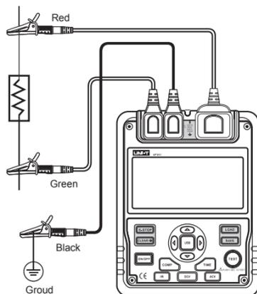
Figure 5. Insulation Resistance Measurement
