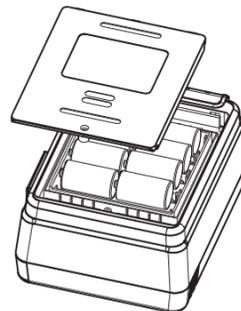
Figure 8. Battery Replacement
