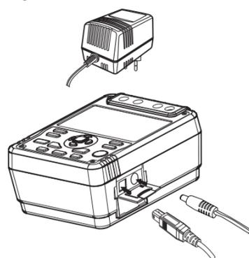
Figure 7. USB Interface Connection
