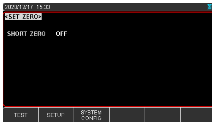
Figure 3-3-2 Short circuit clearing page
