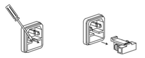
If the fuse was burned out, please replace the same specification fuse with the instrument. The specification fuse with the instrument, see the following table.
