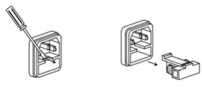
If the fuse was burned out, please replace the same specification fuse with the instrument. The specification fuse with the instrument, see the following table.
