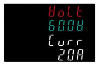
Window 2: the current voltage range, "600V", "300V", "150V", "75V".
