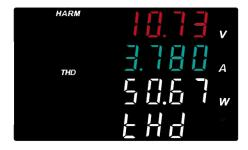
Window 4 displays "tHD" or "or01"~" or50". "tHD" represents the total harmonic distortion; "or01"~" or50" represents the currently selected harmonic times. The display item of window 4 can switch by  $\{ \uparrow \}$  or  $\{ \downarrow \}$ .
