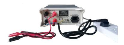
Warning: Before connect with circuit, please make sure the power is cut off to prevent from electric shock.
