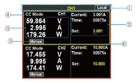
Figure 3-2-1 CC Mode Display Interface (UTL8212)
