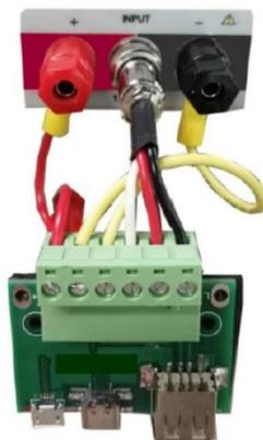
Figure 1-2-3 Connection of Terminal and Quick Charge Test Board (UTL8511C)
