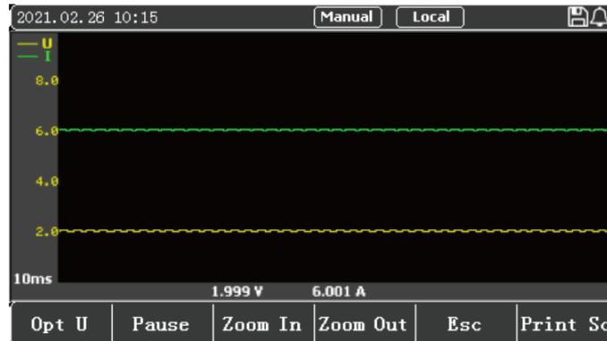
Figure 4-4 Current and Voltage Waveform Display in CV Mode
